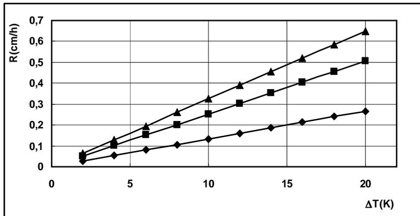
Figure 2. Crystallization rate  $R$  as a function of the difference between the temperature of the melt and that of the airstream  $\Delta T$  in the case of tin (Sn):  $L = 58200$  J/kg,  $\rho = 7300$  kg/m<sup>3</sup>,  $k_b = 0.756$  W/mK,  $k = 59.8$  W/mK,  $\delta = 2$  cm,  $b = 1$  cm —♦—  $\alpha = 20$  W/m<sup>2</sup>K —■—  $\alpha = 50$  W/m<sup>2</sup>K —▲—  $\alpha = 80$  W/m<sup>2</sup>K.
