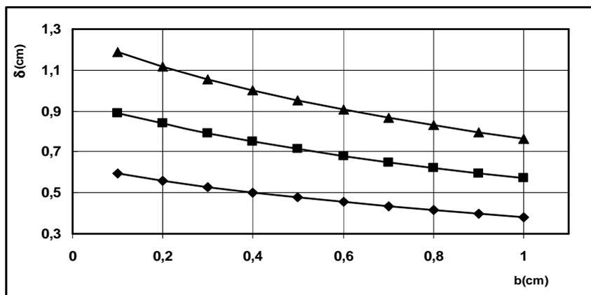
Figure 3. Thickness of crystal layer as a function of the height of the plug  $b$ , in the case of tin (Sn):  $L = 58200$  J/kg,  $\rho = 7300$  kg/m<sup>3</sup>,  $\alpha = 50$  W/m<sup>2</sup>K,  $k_b = 0.756$  W/mK,  $k = 59.8$  W/mK,  $t = 1.5$  h, —♦—  $\Delta T = 10$  K, —■—  $\Delta T = 15$  K, —▲—  $\Delta T = 20$  K.
