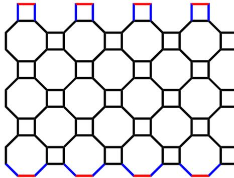
**Fig. 4.** 2-Dimensional Lattice of  $TUC_4C_8[p,q]$  nanotube, with  $p=4$  and  $q=3$
