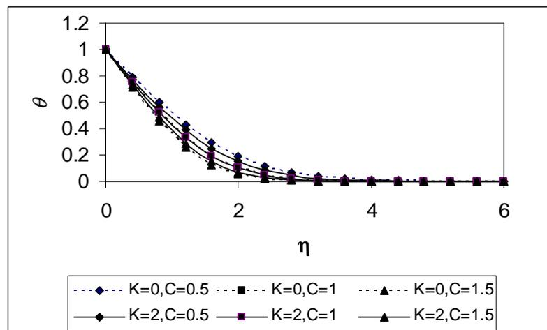
Fig. 2. Effect of the parameters  $C$  and  $K$  on the profile of  $\theta$  ( $Pr=0.7$ ,  $B=0.1$ ).
