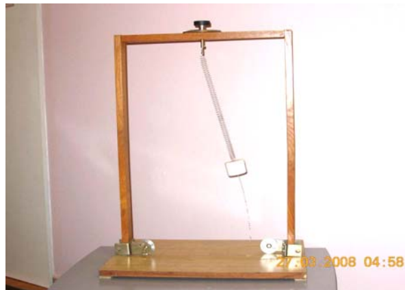
Photograph of the apparatus in action; the instant of maximum horizontal deviation; the flow of water is visible; in this pendulum mode of oscillations, the flow rate depends on the water height in vessel, but otherwise is constant.
