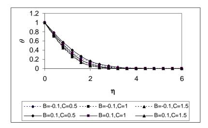
Fig. 4. Effect of the parameters *C* and *B* on the profile of  $\theta$  (*K*=1, *Pr*=0.7)
