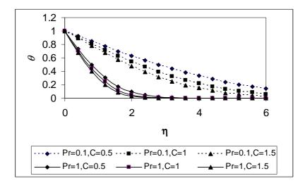
Fig. 3. Effect of the parameters *C* and *Pr* on the profile of  $\theta$  (*K*=1, *B*=0.1).
