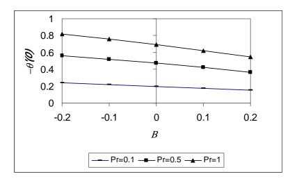
Fig. 5. Variation of the wall heat transfer rate  $-\theta'(0)$  with *B* various values of Pr (*C*=0.5, K=0).
